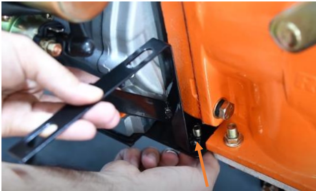
Fit the front wing support.
