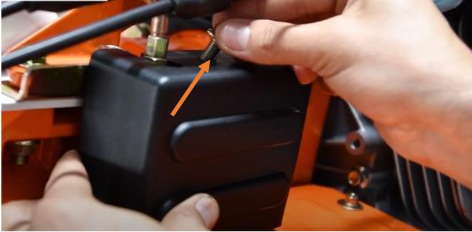
Attach the gearbox trim.
